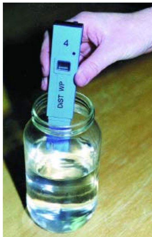
Figure 2. Measuring electrical conductivity with a hand-held meter.
